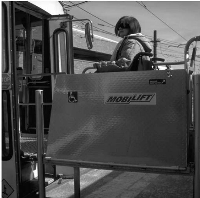
PASSENGER ENTERING GREEN LINE TRAIN VIA MOBILE LIFT
