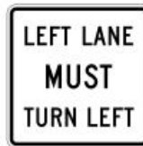
Figure 15 “Left Lane Must Turn Left” (R3-7L) Sign
