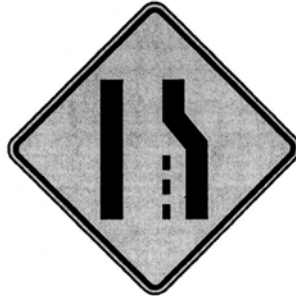
Figure 4-4 “Lane Ends” Warning Sign (W4-2)
