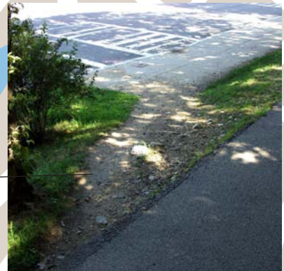
Strong desire lane connecting sidewalk and shared-use path
