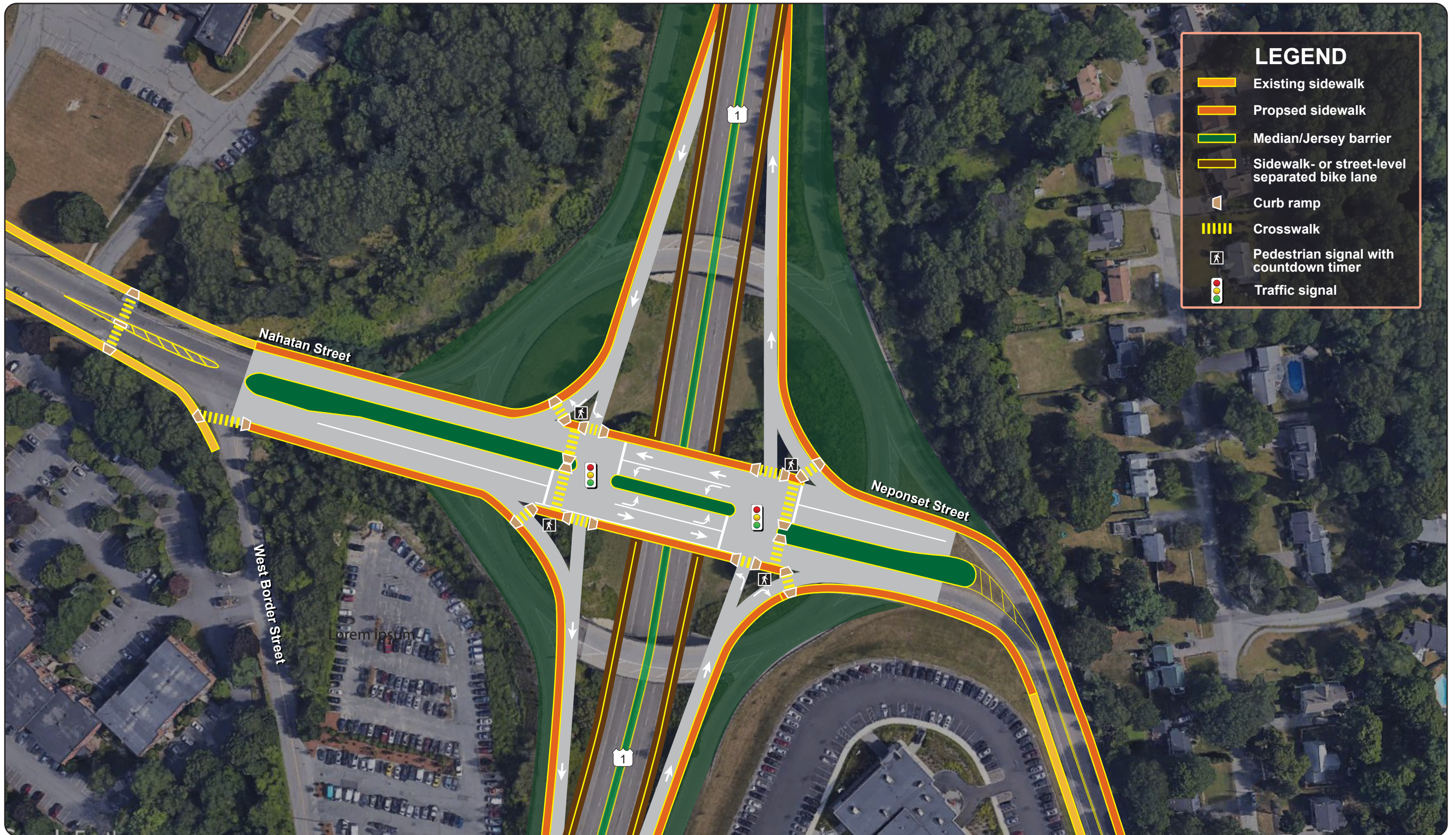
Figure 30 Route 1 at Pendergast Circle: Alternative 2 - Diamond Interchange Concept
