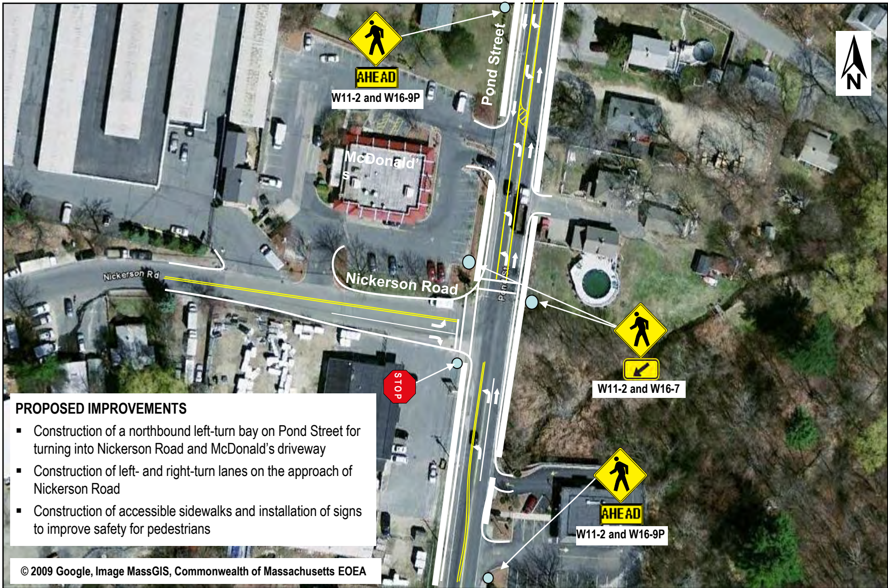
BOSTON REGION MPO FIGURE 6-4 Pond Street and Nickerson Road Intersection: Proposed Improvements Route 126 Corridor Study
